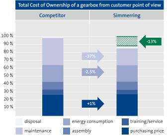
Despite the higher purchasing price of Simmerrings, the Total Cost of Ownership of gearboxes are lower with the usage of FNST products. The savings for Maintenance and Energy are **significant**.
